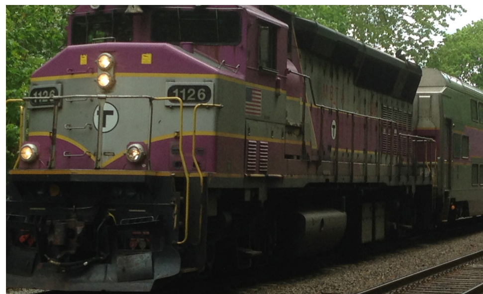
Figure A5.2.6-3: Our optimized NHML alignment will minimize work in the ROW while maintaining the necessary clearance of 17-ft. 9-in. to clear MBTA commuter rail trains in all locations, as well as freight trains.
