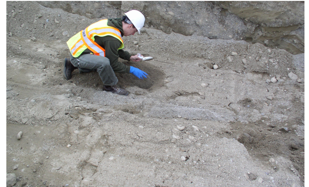
Figure A5.2.8-4: Excavated soils will be identified and pre-classified according to the EMMP.
