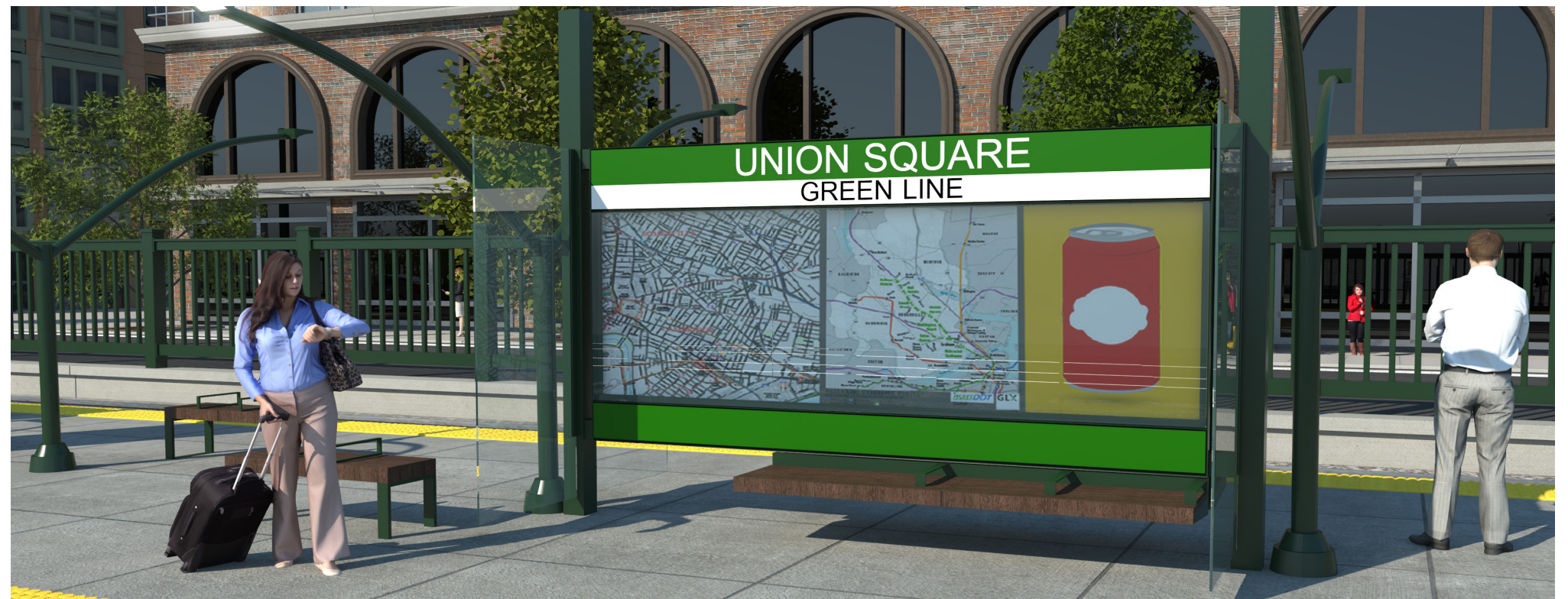
Figure A5.2.4-6: Standard platform signage showing overall MBTA System map, Green Line map, and a third panel that features advertising or other MBTA information signage. This arrangement is similar to the Customer Assistance Area (“CAA”), which replaces the ad panel with an emergency phone.
