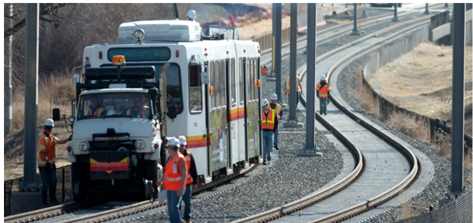
Figure 3.3-1. Rail Line Testing. GLX Constructors' team members support dynamic envelope testing in Denver, Colorado.
