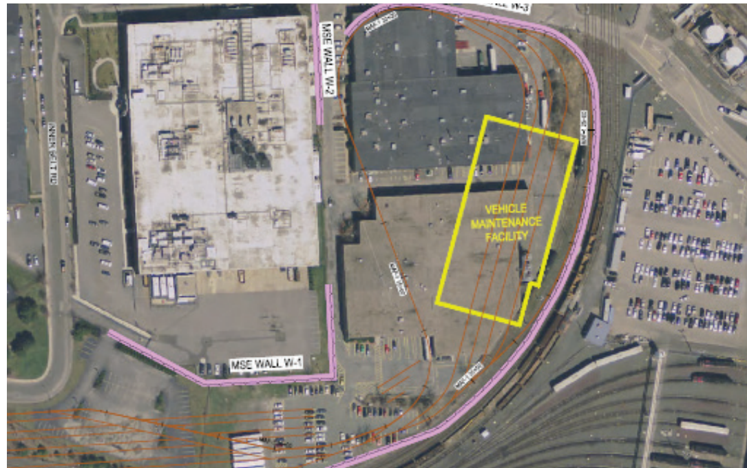
Figure 4.2-10. Approximate Limits of MSE Retaining Walls at the Vehicle Maintenance Facility. MSE walls around the VMF facility allow for the site grade to be raised out of the flood plain and to maximize the use of available space for train storage.
