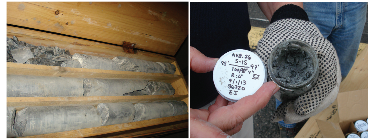
Figure 4.2-19. Variability in Bedrock quality. These photographs demonstrate the extreme variability of the quality of the bedrock. The photo on the left shows competent rock core, and the photo on the right is a sample of rock that was obtained with a standard split spoon soil sampling device.
