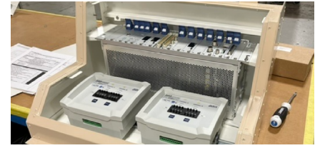
Central equipment enclosure FAI unit
