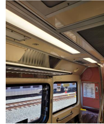
LED Lighting replaced Fluorescents
