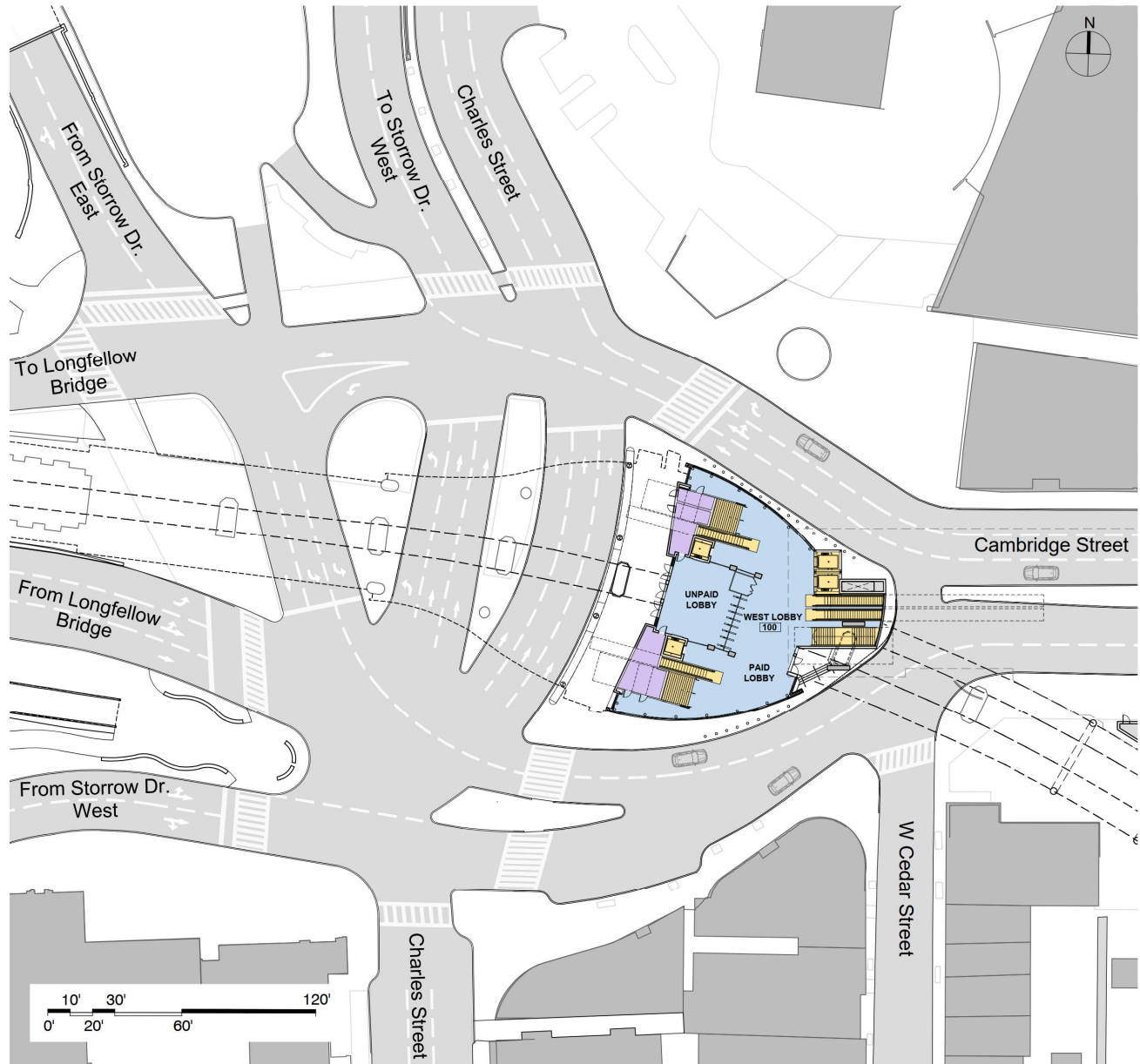
Figure 9-17. Existing Sidewalks, Crosswalks and Pedestrian Access
